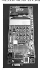
port allows this board to act as a bridge between a PC and a CAN Network. A Windows **CAN-NET** based monitor program can be downloaded from our web site. Microchip PIC16F874 microcontroller supplies the brains. An ICD (In Circuit Debugger) port allows for in-circuit programming and debugging of software when used with the ICD Module (905501). This board may be used as a standalone module or installed in our **Design Center** (905000).
